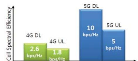
Figure 1. Cell spectral efficiency in 5G networks (Source: 5G Forum)
